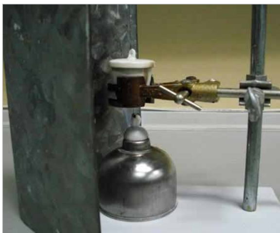
Figure 1. (left) A simple ethanol burner for the calcination process and (right) sketch of the simple ethanol burner setup.
